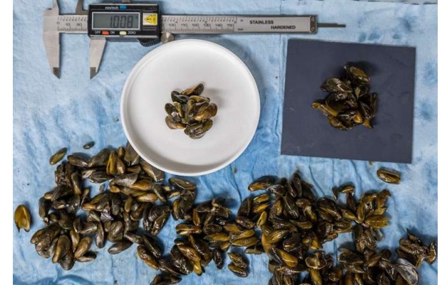
Golden mussel mobile lab staff perform hot water immersion studies to determine the minimum duration and temperature to kill adult mussels.
